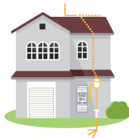
On building ground lead
